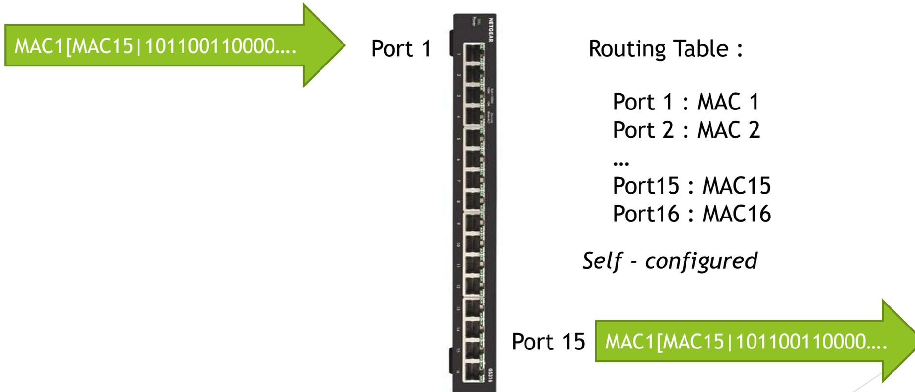
Be carefull, switches are have a max bandwidth or speed in Bytes / s (ex. 100Mb/s, 1Gb/s, 10GB/s ...)
