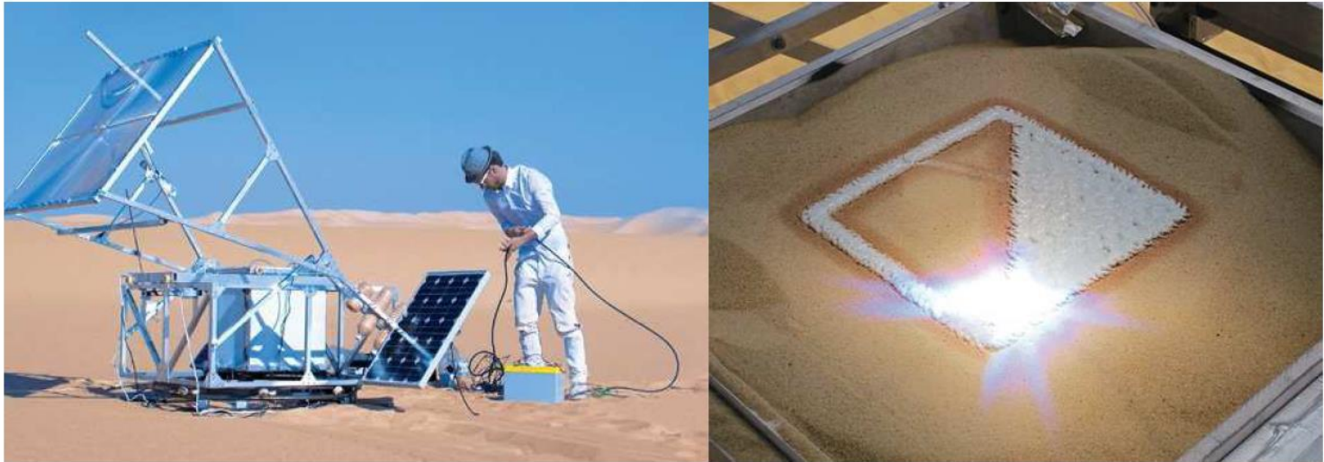
Markus Kayser's "Solar Sinter" 3D printer
