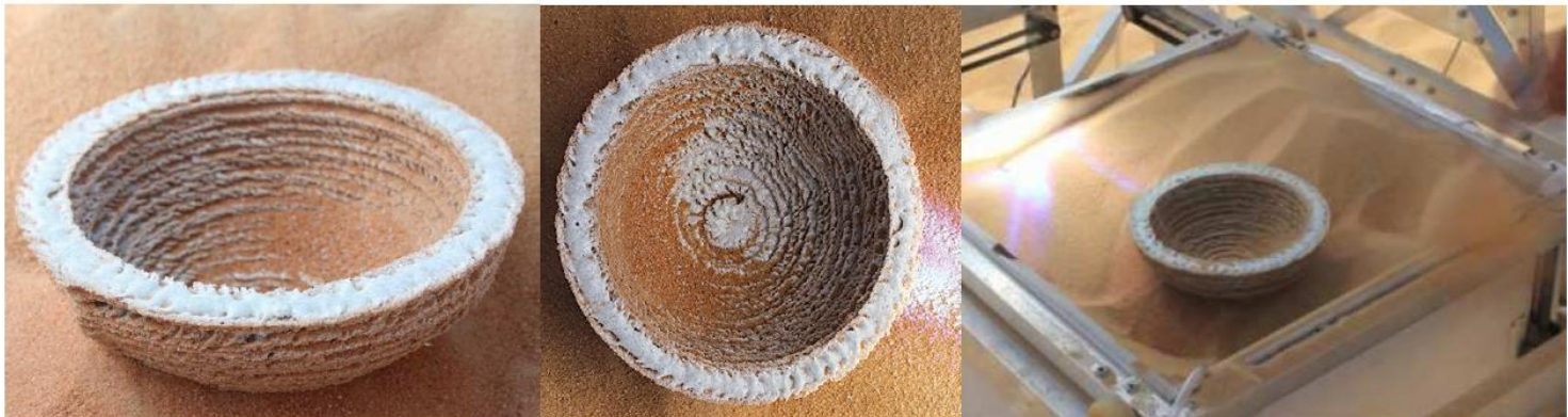
Markus Kayser's "Solar Sinter" 3D printer
