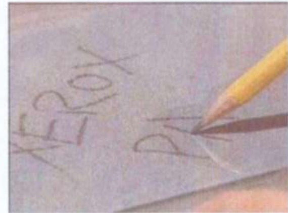
An electronically charged pencil rotates the "pixels"
