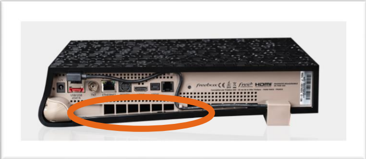
Integrated switch (ex. freebox)
